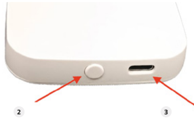
2 Botón Reset Botão Reset / Bouton Reset / Reset Button 3 Conector micro-USB Conector micro-USB / Connecteur micro-USB / Micro-USB connector
